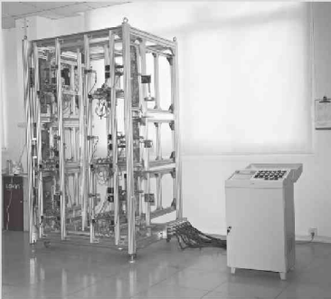
Multiple Cycle Test For Complete Set (Max. test 16 sets at the same time)
